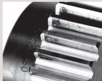
Poor tooth contact and pitting
