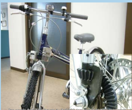
The world's first EMT Bicycle by SHIBUO (includes KHK stainless gears)
