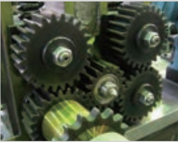
SS spur gears used for wire feeder
