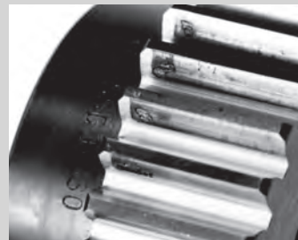
Poor tooth contact and pitting
