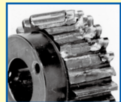
Example of defacement due to insufficient surface durability
