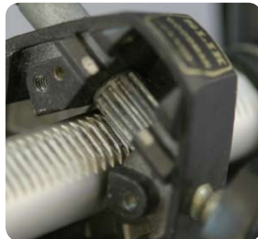
A round rack and a pinion
