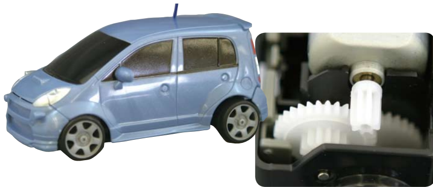
Gears transmitting power and motion to the tires.
