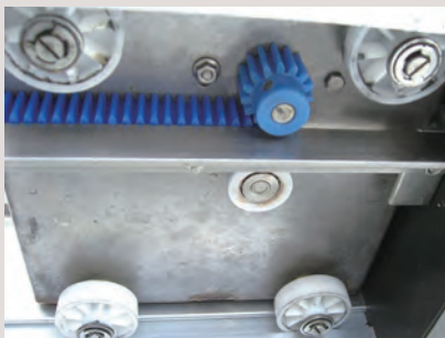
PR plastic rack used for feeding Long Strip Cutter
